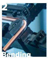
Bending - A wide range of latest generation bending machines allows CFI to shape pipes up to a diameter of 133 x 3
